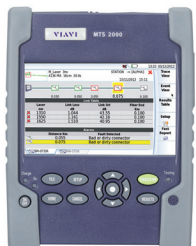
T-BERD/MTS-2000 one-slot handheld modular platform for testing fiber networks
